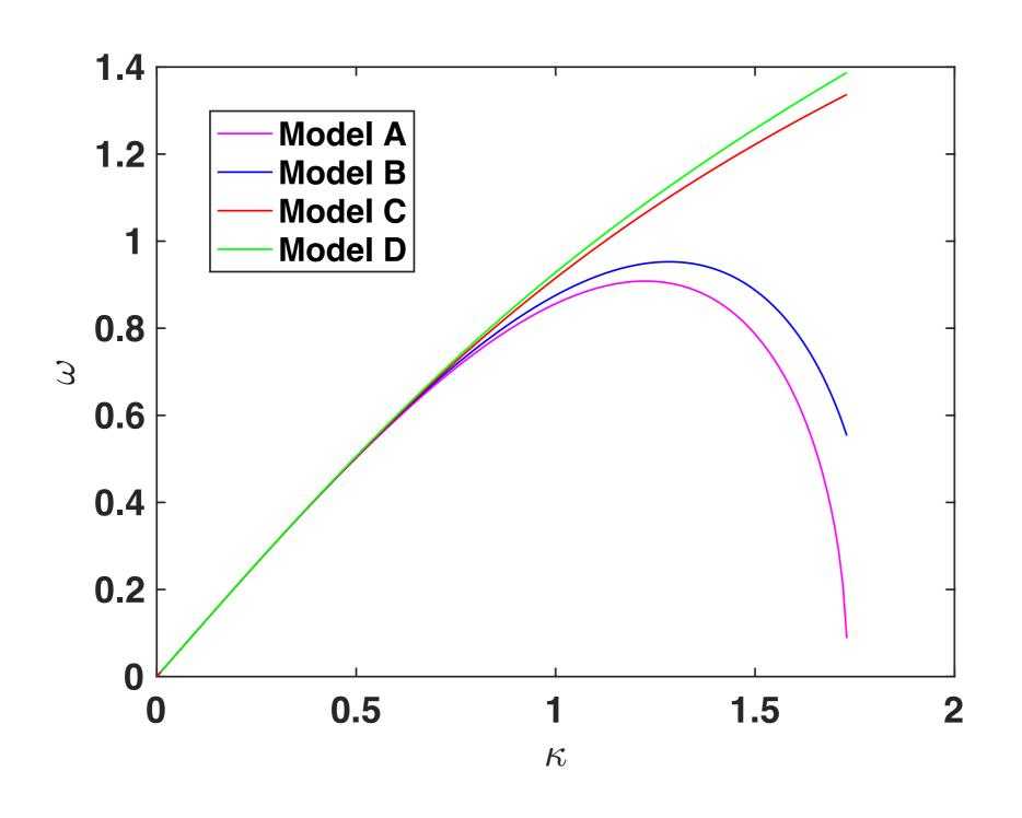
$$\omega^{SystemA}(\bar{\eta},k) = \bar{u}k + k\sqrt{(1+\bar{\eta})\left(1-\frac{1}{3}k^2\right)}$$
